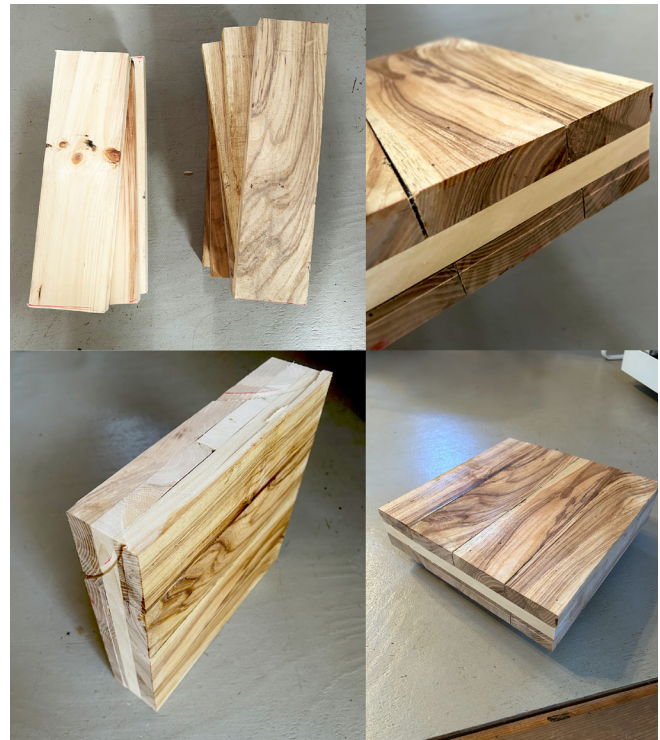
Figure 3. Student made hardwood-CLT sample. Nicholas Brinen, JMU.
